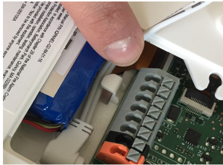
Route the wire behind the retainer clip
