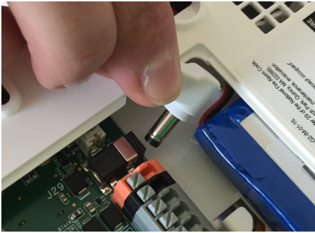
Plug in the power connector
